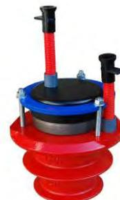
The cap is made up of a cover equipped with a sealing gasket fixed to the casting by means of suitable anchorages which vary in length and size depending on the several applications. A special closing disc tightens the sealing gasket and the cap to the grouting. The disc allows to turn the cap into the most suitable position to allow all the air to come out of the vent tube.
