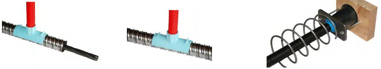
The rear connection guarantees a proper protection of the wire strand without polyvinyl chloride in the area of connection to the anchorage. The unbonded application can be carried out with a metallic sheath and a polyethylene sheath. Sheaths are provided with proper connections for grouting and vent to guarantee a correct grouting after tensioning.
