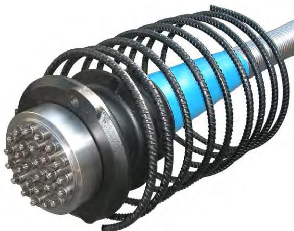
The "M" series active anchorage is made of the following parts: casting, anchor plate, wedges and connection in H.D.P.E. to connect the casting to the metallic or polyethylene sheath. Castings have a turned plane for the plate, holes for connection to cap and formwork and a threaded grouting hole. Castings are in spheroidal cast iron EN-GJS 500-7 EN-JS-1050, which offers a high resistance to stress. Being weldable, it guarantees the maximum safety during installation.
