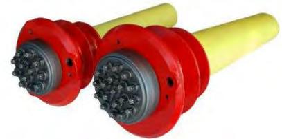
**$M_{EP}^{D\text{®}}$  anchorage in D protection for internal bonded post-tensioning, made of: casting protected with epoxy coating, anchor plate with wedges, polyethylene connection, protection cap, wedges and polyethylene corrugated sheath. The permanent protection cap allows to protect the anchorage by restraining the grouting and by preventing infiltration into the protection cement over time. The anchorage is protected against corrosion with D level.**
