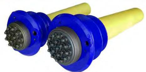
**$MX^E\text{®}$  anchorage in E protection for internal bonded post-tensioning, completely encapsulated in polyethylene, made of casting externally protected with polyethylene, anchor plate with wedges, polyethylene connection, grease-grouted protection cap, wedges and polyethylene corrugated sheath. The permanent protection cap allows to protect the anchorage by filling it with grease, which is a further protective barrier. The anchorage is protected against corrosion with E level.**
