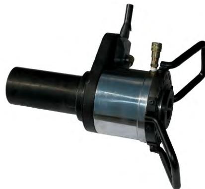
Tightening is by way of chain transmission (inside the jack) driven by a special lever. The lever is supplied with a special device that permits both nut unscrewing and screwing. The chain connects the gears that allow the tightening of the nut; the assembly is protected by a robust casing.
