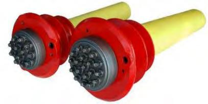
**$M_{EP}^{C\text{®}}$  anchorage in C protection for internal bonded post-tensioning, made of: casting protected with epoxy coating, anchor plate with wedges, polyethylene connection, protection cap, wedges and galvanized metallic corrugated sheath. The permanent protection cap allows to protect the anchorage by restraining the grouting and by preventing infiltration into the protection cement over time. The anchorage is protected against corrosion with C level.**
