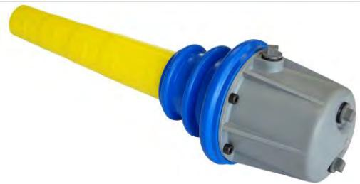
*The application of X anchorages may be unbonded or bonded with grouting of cement or grease. The encapsulation of the whole anchorage with minimum 3mm polyethylene thickness allows a strong encapsulation of the device, which prevents corrosive agents from affecting its durability and effectiveness. The effectiveness of the system is completed by the use of polyethylene corrugated sheaths which guarantee the encapsulation of the whole cable.*
