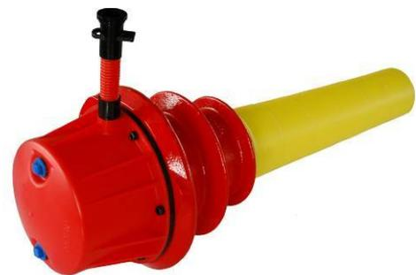
The "M" series active anchorage is made of the following parts: casting, anchor plate, wedges and connection in H.D.P.E. to connect the casting to the metallic or polyethylene sheath. Castings have a turned plane for the plate, holes for connection to cap and formwork and a threaded grouting hole. Castings are in spheroidal cast iron EN-GJS 500-7 EN-JS-1050, which offers a high resistance to stress. Being weldable, it guarantees the maximum safety during installation.
