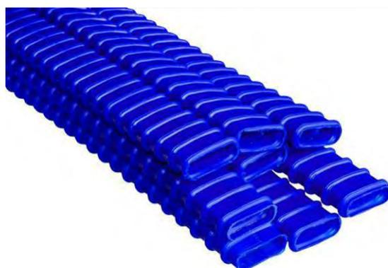
*SPE-78x25x2 mm. polyethylene sheaths are made of extruded H.D.P.E. according to the FIB Specification, in bars with a length from 5.8 m. to 11.8 m. They are blue with a heat-shrinking sleeve on each connection.*
