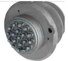
**$ME^M$  anchorage in M protection from external unbonded post-tensioning, made of casting submerged into concrete, anchor plate with wedges, painted steel connection, cement-grouted protection cap, wedges and use of bare strands. The protection cap allows to protect the anchorage with a cement filling. The anchorage can be replaced over time if required.**
