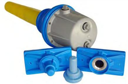
*X series anchorages, both single and multi-strand, are encapsulated with polyethylene in order to guarantee unlimited durability and resistance against corrosion provided the devices are properly installed. A layer of polyethylene covers the whole anchorage, allowing a grouting of cement or grease inside it.*
