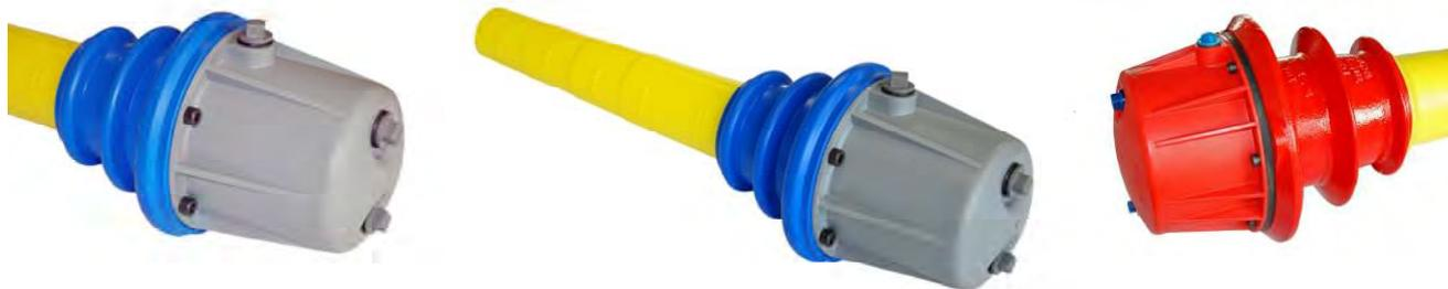
The DD-KP cap is made of polyethylene and together with a MEP or MX anchorage guarantees a double protection to corrosion. The DD-KP cap is provided with plugs to guarantee a correct grouting and vent when filling it.
