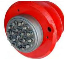
**ME<sub>EP</sub><sup>N®</sup> anchorage in N protection from external bonded post-tensioning, made of casting protected with epoxy coating submerged into concrete, anchor plate with wedges, steel connection protected with epoxy coating, cement grouted protection cap, wedges and the use of bare strands. The protection cap allows to protect the anchorage with a cement filling. The anchorage can be replaced over time if required.**
