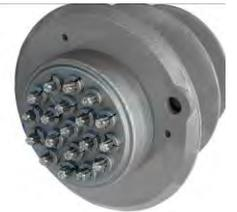
**$ME^L$  anchorage in L protection from external bonded post-tensioning, made of casting submerged into concrete, anchorage with wedges, painted steel connection, cement-grouted protection cap, wedges and use of bare strands. The protection cap allows to protect the anchorage with a cement filling. This application is the simplest among those which can be replaced over time.**
