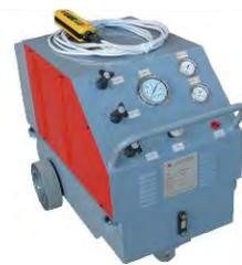
*(Tensioning of TTM and M multi-strand anchorages)*
