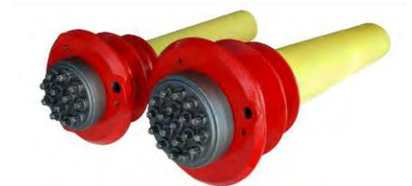
**$M_{EP}^{D\text{®}}$  anchorage in D protection for internal bonded post-tensioning, made of: casting protected with epoxy coating, anchor plate with wedges, polyethylene connection, protection cap, wedges and polyethylene corrugated sheath. The permanent protection cap allows to protect the anchorage by restraining the grouting and by preventing infiltration into the protection cement over time. The anchorage is protected against corrosion with D level.**
