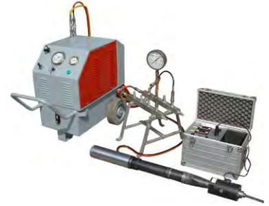
(Dynamometer for jack calibration)
