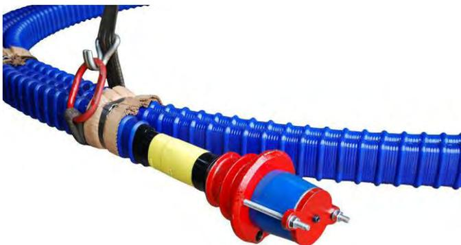
*Cables are provided with proper fastenings that allow to lift and handle them without damaging the sheath, which is made of polyethylene to allow rolling up. Sheaths are seamed by means of heat-shrinking elements in order to guarantee continuity and seal.*
