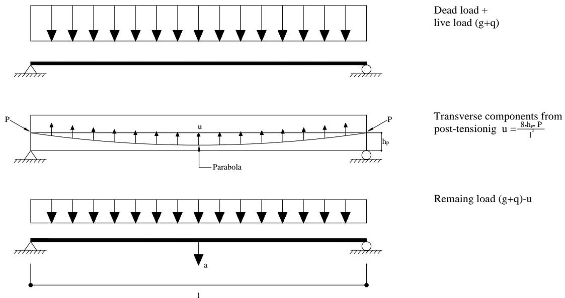
Principle of the equivalent cable
