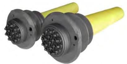
$M$  anchorage for normal internal bonded post-tensioning, made of: casting, anchor plate with wedges, polyethylene connection, wedges and metallic corrugated sheath. The anchorage is protected against corrosion with A level.
