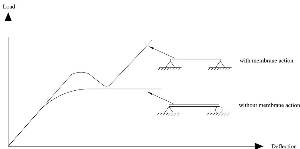
Effect of the bending stress on the slab load-bearing capacity
