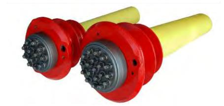
**$M_{EP}^{C\text{®}}$  anchorage in C protection for internal bonded post-tensioning, made of: casting protected with epoxy coating, anchor plate with wedges, polyethylene connection, protection cap, wedges and galvanized metallic corrugated sheath. The permanent protection cap allows to protect the anchorage by restraining the grouting and by preventing infiltration into the protection cement over time. The anchorage is protected against corrosion with C level.**
