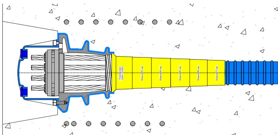
The resulting anchorage is used together with the casting versions **MEP**<sup>®</sup> and **MX**<sup>®</sup> encapsulated and protected, in particular in the most complete version **MX**<sup>®</sup> completely encapsulated in polyethylene.
