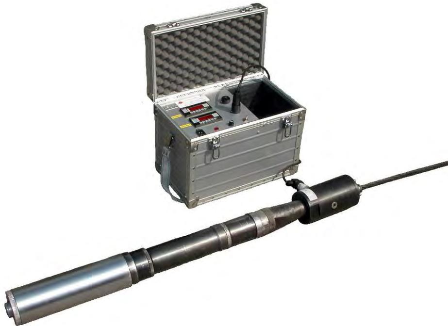
The dynamometer is provided with a calibration certificate issued by a **S.I.T.** centre or an authorized laboratory with a six month validity.
