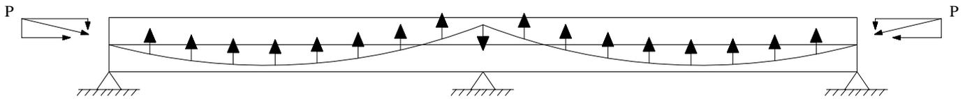
Transverse components and axial forces resulting from the application of post-tensioning
