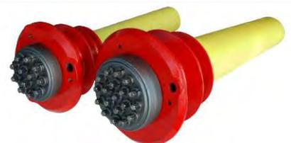
$M_{EP}^{B\text{®}}$  anchorage in **B** protection for internal bonded post-tensioning, made of: casting protected with epoxy coating, anchor plate with wedges, polyethylene connection, wedges and galvanized metallic corrugated sheath. The anchorage is protected against corrosion with F level.
