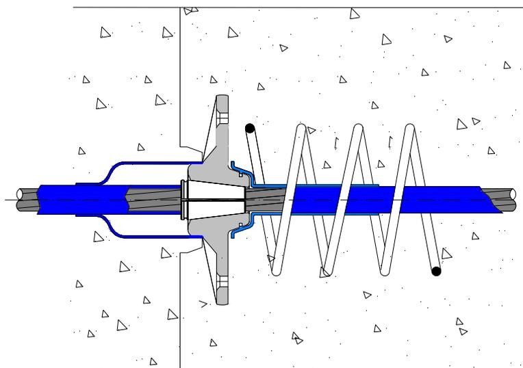
**2.16 - 1E15 unbonded through anchorage with DD 1095GK gasket**
