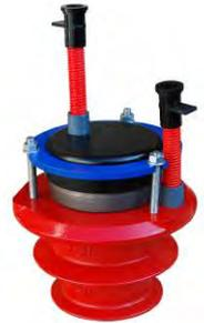
The cap is made up of a cover equipped with a sealing gasket fixed to the casting by means of suitable anchorages which vary in length and size depending on the several applications. A special closing disc tightens the sealing gasket and the cap to the grouting. The disc allows to turn the cap into the most suitable position to allow all the air to come out of the vent tube.
