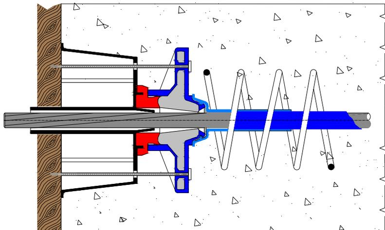
*1EX15 anchorage with rectangular DD-1097A pocket former and DD 1096GK sealing gasket directly applied onto the formwork.*
