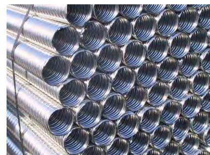
*ST metallic sheaths are available in different versions. They are made of crimped sheet EN 10139 - 1999. They can be galvanized. Sheaths are available in bars having a length of 5.8 m. They are all provided with a sleeve screwed onto each bar.*
