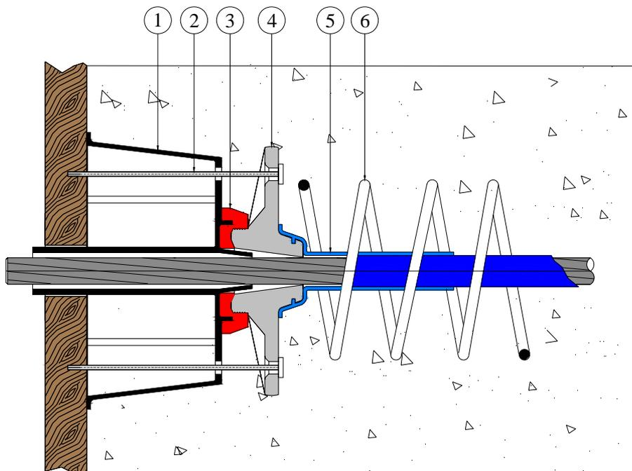
The 1E15 unbonded active anchorage with DD-1097A rectangular pocket former and DD 1095GK sealing gasket is made of the following parts: **Ref. 1** DD-1097A rectangular pocket former, **Ref. 2** fixing screws, **Ref. 3** DD 1095GK sealing gasket **Ref. 4** 1E15 steel anchor plate, **Ref. 5** rear connection and **Ref. 6** spring steel reinforcement,
