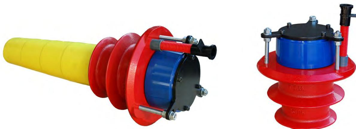
The “D” series active anchorage is made of the following parts: casting, preassembled D anchor plate, wedges and connection in H.D.P.E. to connect the casting to the metallic sheath. Castings have a turned plane for the plate, holes for connection to cap and formwork and a threaded grouting hole. Castings are in spheroidal cast iron EN-GJS 500-7 EN-JS-1050, which offers a high resistance to stress. Being weldable, it guarantees the maximum safety during installation.
