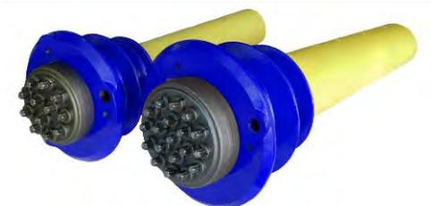
**$MX^{E\text{®}}$  anchorage in E protection for internal bonded post-tensioning, completely encapsulated in polyethylene, made of casting externally protected with polyethylene, anchor plate with wedges, polyethylene connection, grease-grouted protection cap, wedges and polyethylene corrugated sheath. The permanent protection cap allows to protect the anchorage by filling it with grease, which is a further protective barrier. The anchorage is protected against corrosion with E level.**
