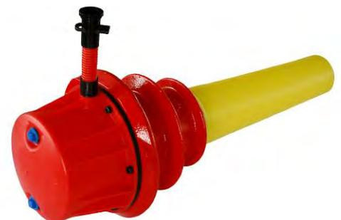
The “M” series active anchorage is made of the following parts: casting, anchor plate, wedges and connection in H.D.P.E. to connect the casting to the metallic or polyethylene sheath. Castings have a turned plane for the plate, holes for connection to cap and formwork and a threaded grouting hole. Castings are in spheroidal cast iron EN-GJS 500-7 EN-JS-1050, which offers a high resistance to stress. Being weldable, it guarantees the maximum safety during installation.
