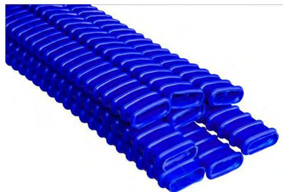
*SPE-78x25x2 mm. polyethylene sheaths are made of extruded H.D.P.E. according to the FIB Specification, in bars with a length from 5.8 m to 11.8 m. They are blue with a heat-shrinking sleeve on each connection.*
