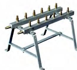
By means of a manifold, all the hydraulic pumps can be connected to several tensioning jacks. The **DD-MF** manifold is designed with 4, 6 or 10 hydraulic outputs under isopressure, it is made of galvanized steel and can be completely disassembled. The upper connections are for jacks, the side connections are for **TTM pumps**
