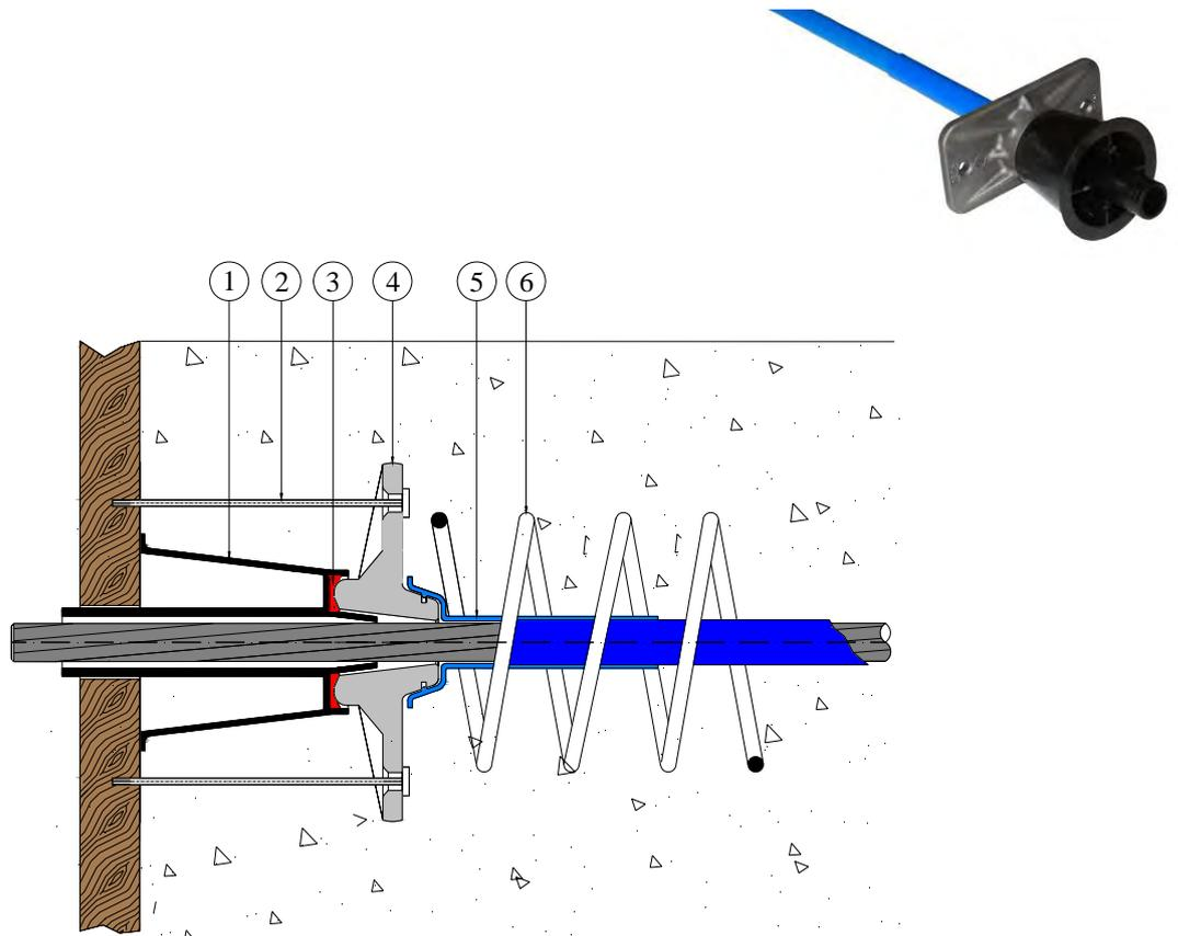
The 1E15 unbonded active anchorage with DD 7099B truncated cone pocket former and DD 7025 sealing gasket is made of the following parts: **Ref. 1** DD-7099B truncated cone pocket former, **Ref. 2** fixing screws, **Ref. 3** DD 7025 sealing gasket, **Ref. 4** 1E15 steel anchor plate, **Ref. 5** rear connection and **Ref. 6** spring steel reinforcement,
