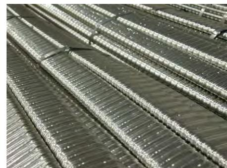
*SL metallic sheaths are available in different versions. They are made of crimped sheet EN 10139 - 1999. They can be galvanized. Sheaths are available in bars having a length of 5.8 m. They are not all provided with a sleeve screwed onto each bar obtaining their connection by overlapping.*
