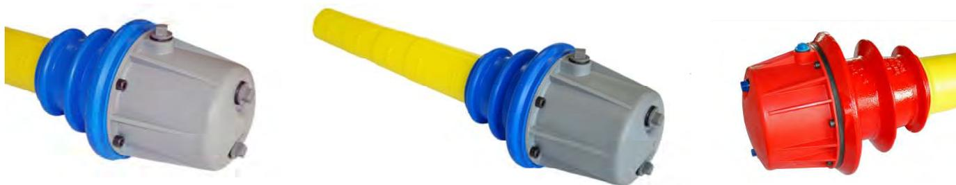
The DD-KP cap is made of polyethylene and together with a MEP or MX anchorage guarantees a double protection to corrosion. The DD-KP cap is provided with plugs to guarantee a correct grouting and vent when filling it.
