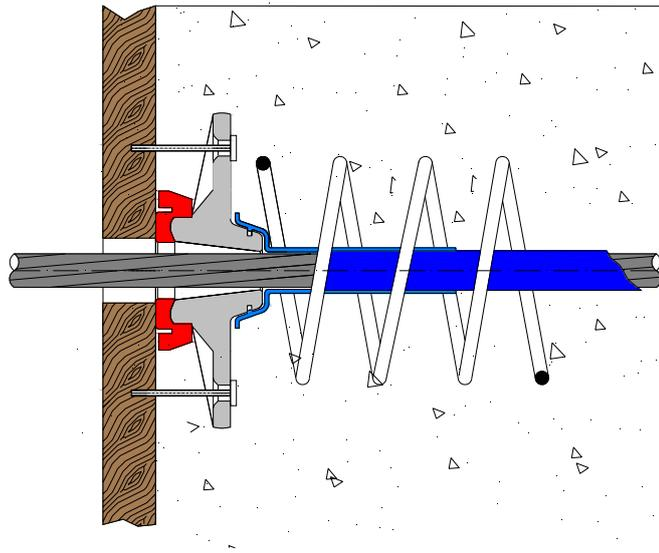
**2.17 - 1EX15 unbonded anchorage with DD 1096GK gasket**
